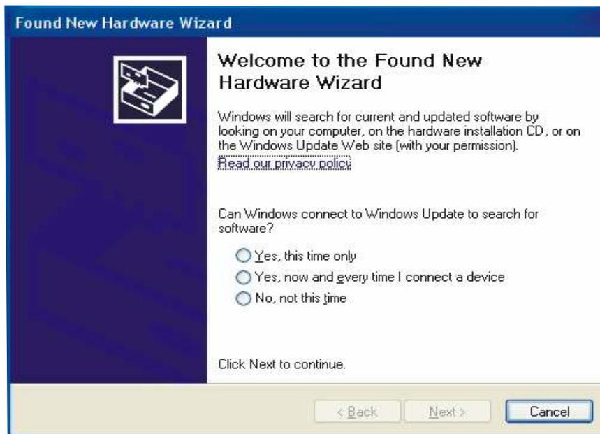
**Step 2.** Install the Synway device driver ShCti4.7 in the system from the installation CD. Insert the CD into the CD-ROM drive and run the application file
