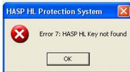
**Solution:** This error appears when HASP HL Key is not inserted into the USB port of the computer.
