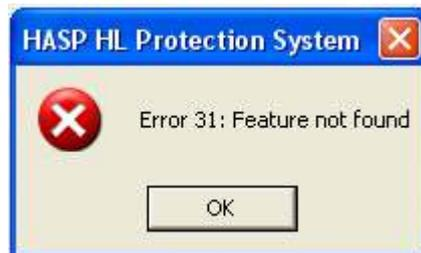
**Solution:** This error happens when the HASP HL Key connected to the USB port of the computer does not have license to run Xtend Voice Logger.
